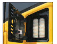
External air conditioner filter
