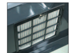
Internal air conditioner filter
